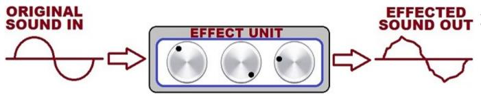
An Effect Unit takes a sound (input) and creates an effected version of it (output).
